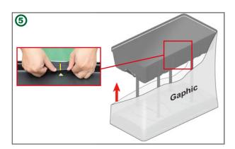
Set up grpahic upgrade,pay attention that mark line in graphic should match with the triangle mark in the talbe top.
