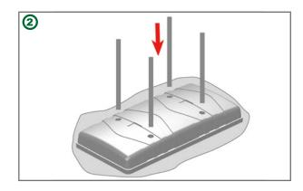
Put the cap of case in the middle of graphic and install vertical pipes.
