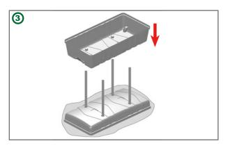
Install body of case well with vertical pipes.
